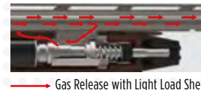
Gas Release with Light Load Shell
